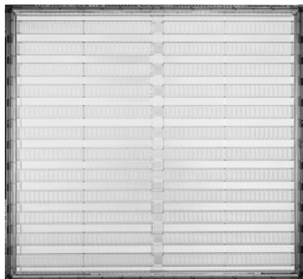
Figure 1.2 A field-programmable gate array chip (courtesy of Altera Corp.).
